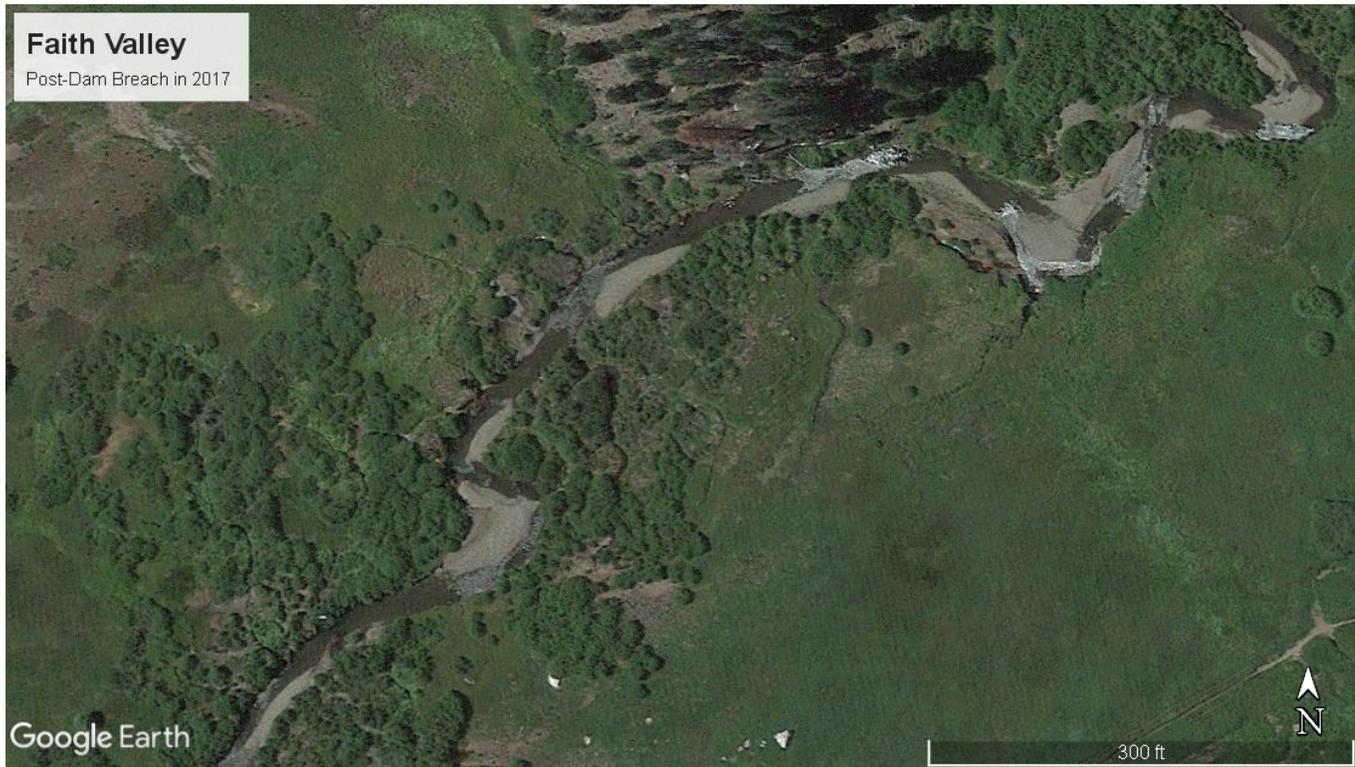
Figure 16. Post-Dam breach in 2017. Note the huge amount of sediment that was trapped behind the dam and was then washed downstream and deposited after the breach. These dynamics of dam building, inundation, breaching, sediment capture and distribution, and willow cropping are essential meadow processes that leave distinct visual remains.
