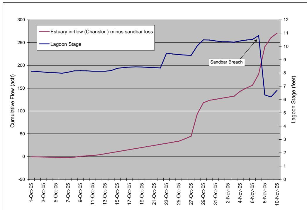
**Figure 3.1.7** Lagoon water surface elevations pre- and post-breach 2005 as they relate to stream flows. The sandbar breached on November 8<sup>th</sup>. Cumulative inflows were calculated to be approximately 180 acre feet at the time of breach. Given the level of approximation in these estimates, this correlates well with the volume of 135 ac ft needed to fill the lagoon.
