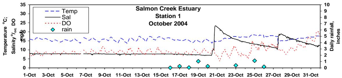
**Figure 3.3.2** October, 2004 records show two peaks of saline water entering the lower estuary from upstream. These peaks followed rain events; the beach berm has not been breached to allow tidal waters to enter the estuary.
