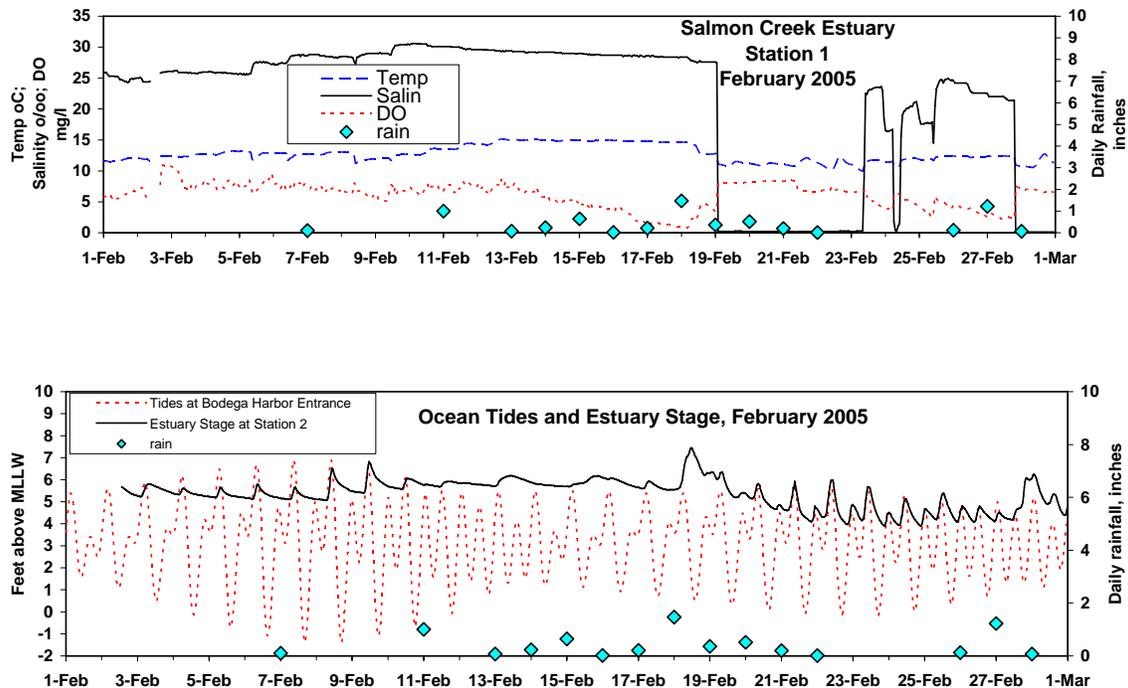
Figure 3.3.5 Water quality and water surface elevation conditions shown with corresponding tidal and rain records.
