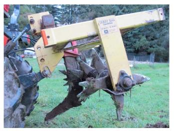
*Close-up of the special blade and rotating tines on the keyline plow*
