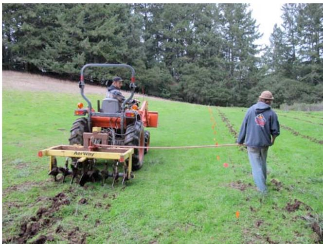
*Using the keyline plow to cut keylines just off contour to direct water away from road and towards the forest in the background*
